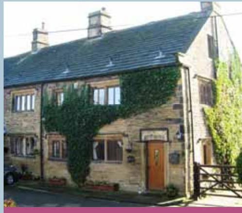
Locally quarried sandstone sits beneath a stone slate roof. Older properties display narrow coursing.
